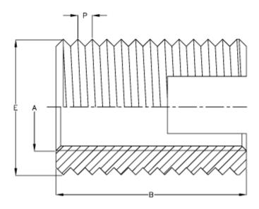
Female thread A = M20 Length B = 27 Male thread E = 26.0 Min hole depth blind hole = 32
